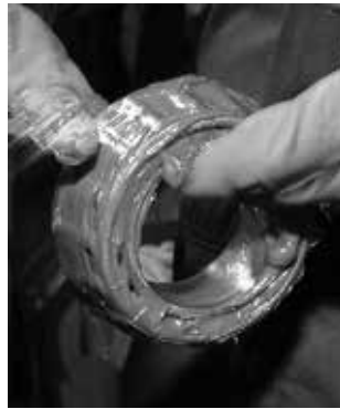
Fig. 23. Grease can easily be packed by hand.
